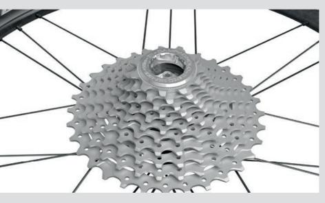
Same cassette width: total compatibility with the current free-hub bodies and the current frames rear chainstays width, obtained with thinner sprockets
