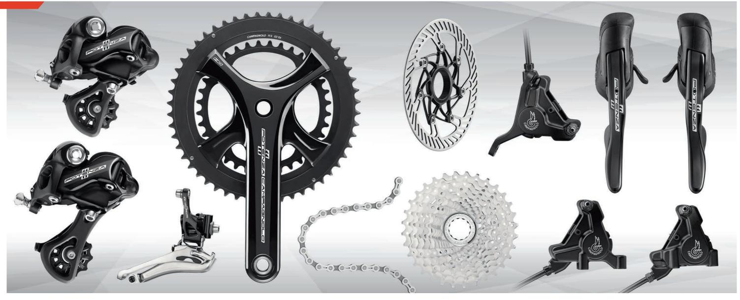
The premium aluminum offering from Campagnolo®, the **Potenza 11™ disc brake** groupset combines the performance of the top end groups with the increased versatility of a rear derailleur capable of incorporating up to 32 tooth
