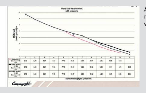
An extra gear makes for more efficient gearing with less gaps
